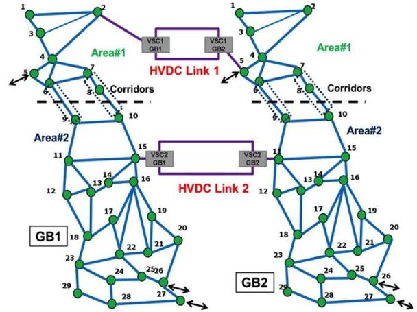
Figure 4: GB1 and GB2 connected through two VSC HVDC links.
