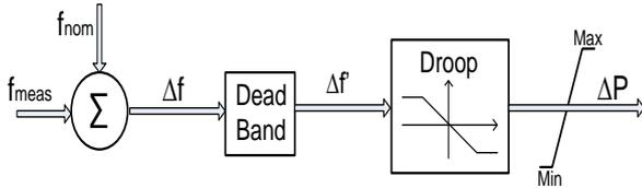
Figure 3: Droop control loop for the rectifier HVDC converter
