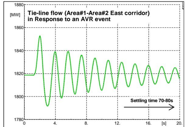
Figure 2: Tie-line flow in Line 8-10 in response to an AVR step change event applied at G18.
