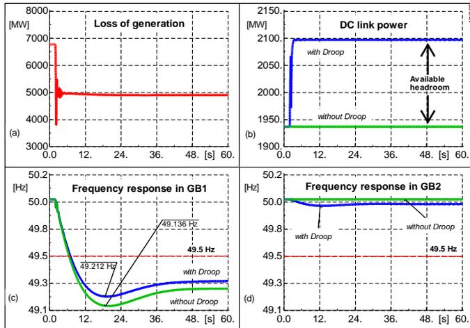
Figure 6: Dynamic performance of the system under a loss of generation event at G15 in GB1. (a) Power flow in G15 in GB1. (b) DC link power in HVDC Link1. (c) Frequency response in GB1. (d) Frequency response in GB2.
