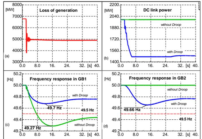
Figure 5: Dynamic performance of the system under a loss of generation event at G15 in GB1. (a) Power flow in G15 in GB1. (b) DC link power in HVDC Link1. (c) Frequency response in GB1. (d) Frequency response in GB2.
