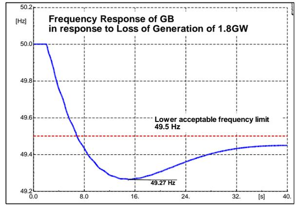
Figure 1: Frequency response of the system after a 1.8GW loss of generation (at G19).
