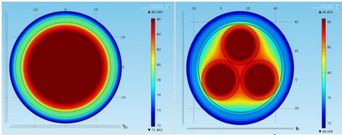
Fig. 1. Heat distribution in the different layers of the 300 mm<sup>2</sup> cables at the maximum current capacity.
