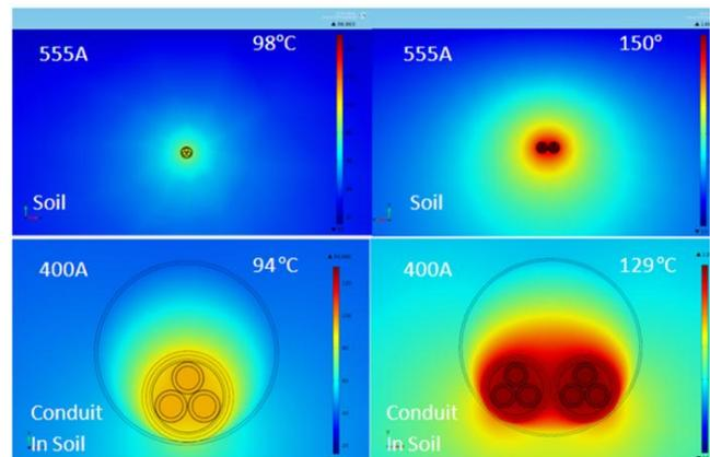
Fig. 3. Heat distribution of the three core cable buried 80cm in different scenarios and different current ratings. Maximum conductor temperature is shown.
