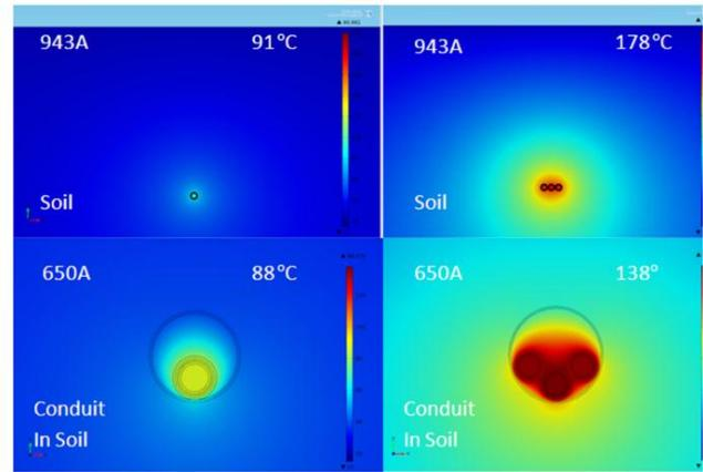
Fig. 2. Heat distribution of the single core cable buried 80cm in different scenarios and different current ratings. Maximum conductor temperature is shown.
