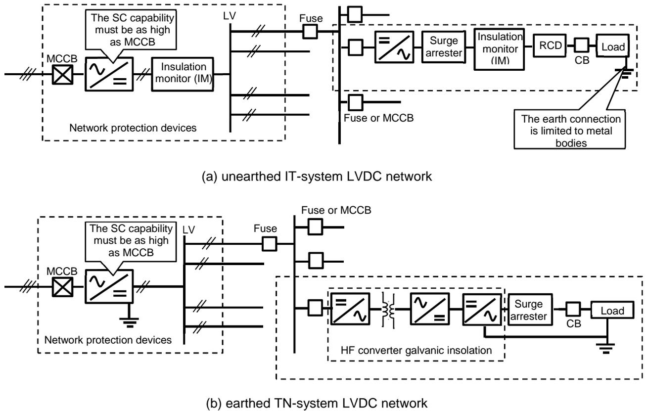
Figure 21: Protection schemes of earthed and unearthed LVDC distribution networks [54]
