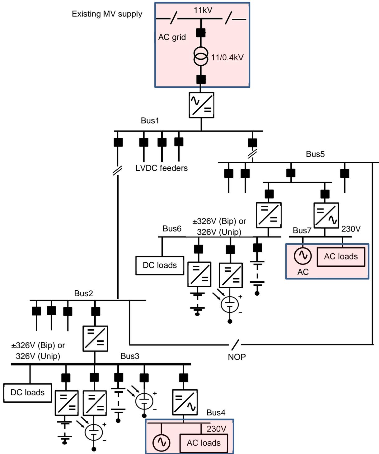
Figure 4: An LVDC network topology example
