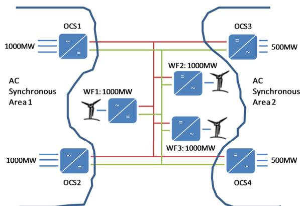
**Figure 4: example DC grid and dispatch of power totalling 2GW to area 1 and 1GW to area 2**
