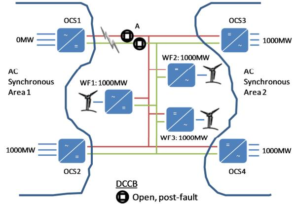
**Figure 7: example DC with DCCBs at location A that succeed in clearing a fault between OSC1 and location A**
