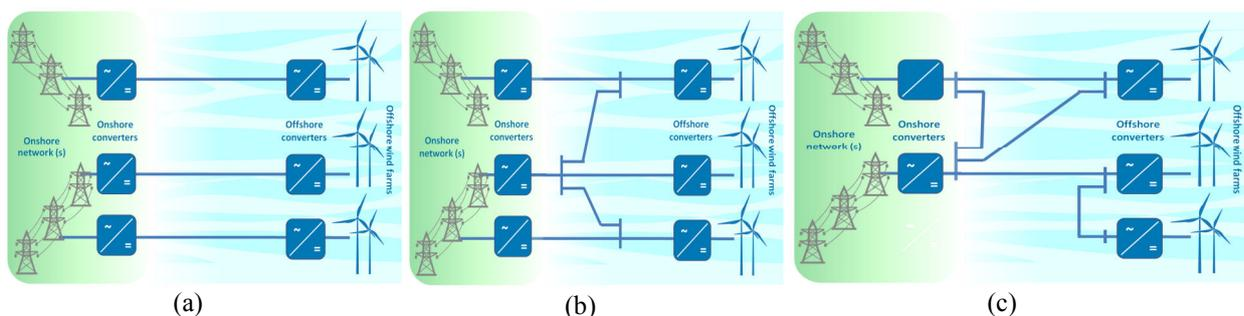
**Figure 3: possible DC offshore network structures: point-to-point, radial and meshed [24]**
