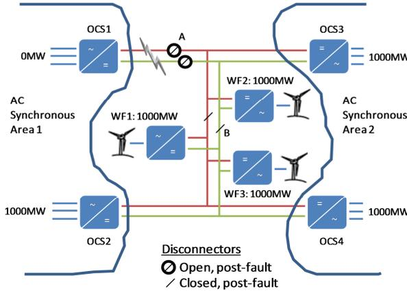
**Figure 6: post-fault reconfiguration of the example DC grid**
