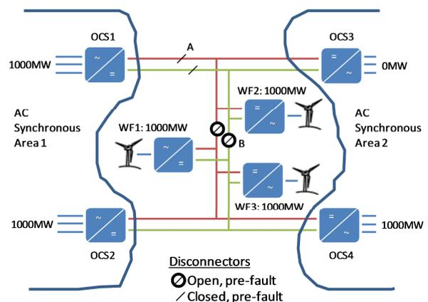
**Figure 5: example DC grid with a pre-fault split introduced at location B**
