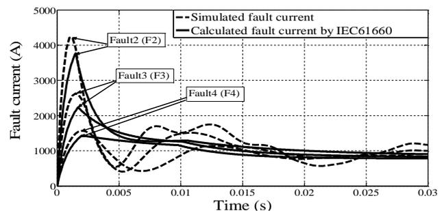
Figure 3: DC remote faults at different locations
