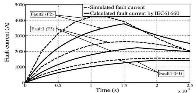
Figure 4: The rise times of DC remote faults
