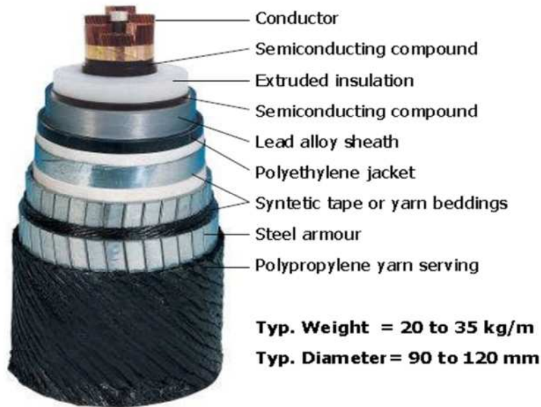
Figure 14 structure of extruded cable [64]
