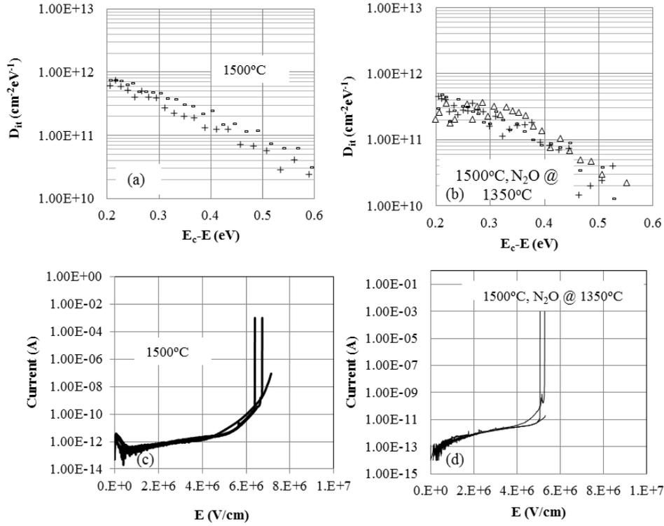
Fig. 1. Typical I-V characteristics of 4H-SiC MOS capacitors with a high-temperature ( $1500^\circ\text{C}$ ) thermal oxidation followed by with/without post-oxidation  $\text{N}_2\text{O}$  annealing at  $1350^\circ\text{C}$ , interface trap density (a-b), and oxide breakdown (c-d).
