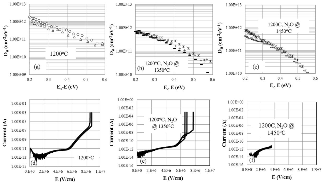
Fig. 2. Typical I-V characteristics of 4H-SiC MOS capacitors with a standard oxidation process ( $1200^\circ\text{C}$  thermal oxidation) and followed by post-oxidation  $\text{N}_2\text{O}$  annealing at  $1350^\circ\text{C}$  and  $1450^\circ\text{C}$ .
