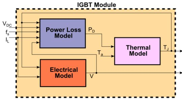
Figure 13. The electro-thermal model of the IGBT module used to study residuals behavior with packaging degradation
