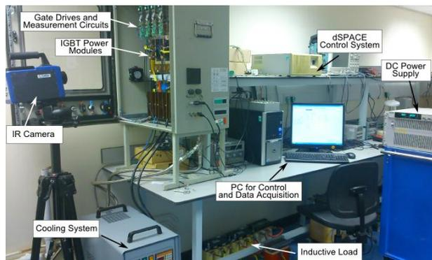
Figure 11. Experimental setup of the full-bridge inverter used to validate the real-time estimate of junction temperature  $T_J$ .
