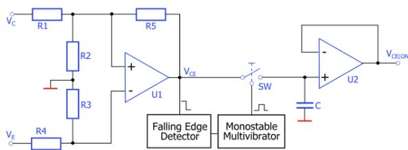
Figure 4. A block diagram of the online measurement circuit of  $V_{CE(ON)}$
