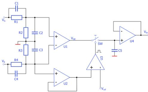
Figure 8. The online measurement circuit of threshold voltage
