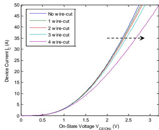
Figure 3. I-V characteristic of a single-chip IGBT module shows change of  $V_{CE(ON)}$  with wire-bond attached.
