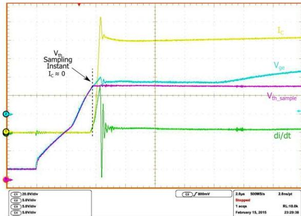
Figure 9. Operating waveforms of  $V_{th}$  measurement circuit during a normal switching cycle of an IGBT. Device current ( $I_C$ ), gate-emitter voltage ( $V_{ge}$ ),  $di/dt$  measured across parasitic inductance ( $di/dt$ ) and measured  $V_{th}$  ( $V_{th\_sample}$ )
