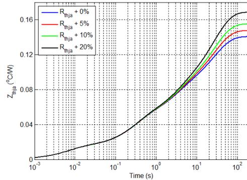
Figure 14. Simulated Thermal Impedances for baseline case ( $R_{thja}+0\%$ ) and degraded cases (5%, 10% and 20%)
