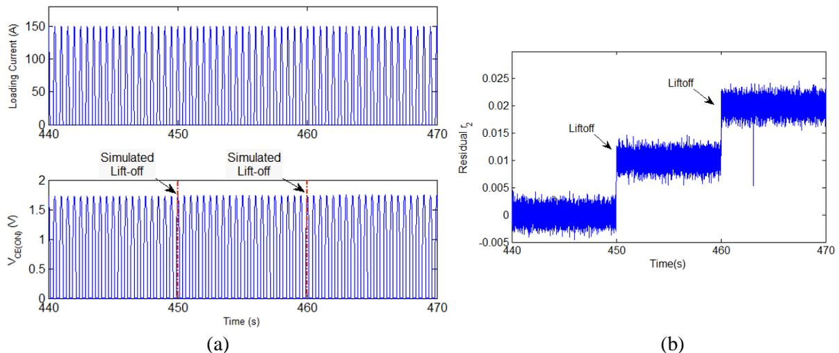
Figure 16. (a) Simulated IGBT loading current and  $V_{CE(ON)}$  in a single phase inverter during wire-bond lift-offs. It is difficult to detect changes in  $V_{CE(ON)}$  due to masking effect of operating conditions. (b) The residual  $r_2(k)$  removes masking effects and reveals changes in  $V_{CE(ON)}$  resulting from wire-bond failures.
