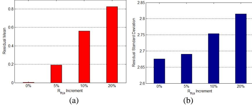
Figure 15. Change of Residual Statistics as a result of thermal degradation. Mean (a) and Standard Deviation (b) both increase with increasing thermal resistance  $R_{thja}$
