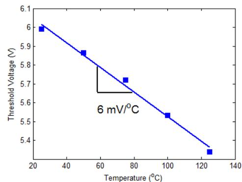
Figure 7. Variation of threshold voltage  $V_{th}$  with temperature as extracted from the transfer characteristic.
