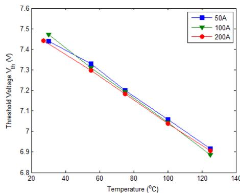
Figure 10. Calibration of threshold voltage with temperature in a double pulse test. Threshold voltage  $V_{th}$  is measured using the proposed circuit.
