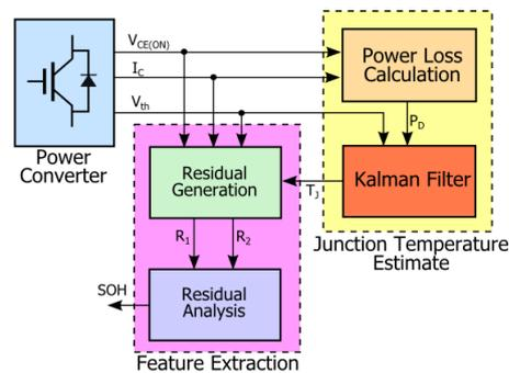
Figure 1. Real-time Health monitoring of IGBT power modules.
