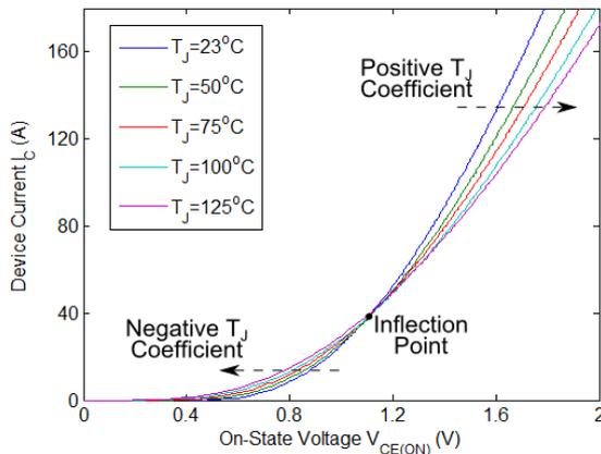
Figure 2. I-V characteristic of a 1.2kV/400A IGBT power module at multiple temperatures explains temperature dependency of the on-state voltage  $V_{CE(ON)}$ .
