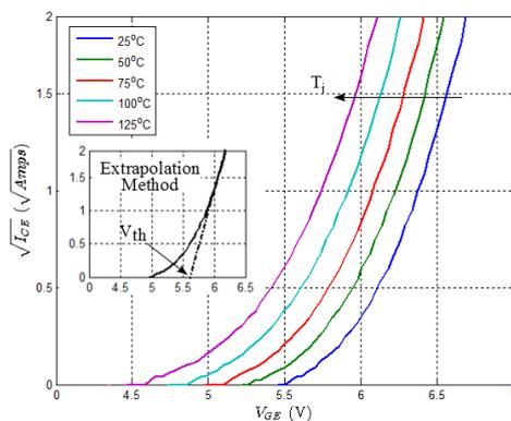
Figure 6. square-root of current vs.  $V_{GE}$  shows variation of threshold voltage at multiple temperatures of 1.2kV/400A IGBT module.
