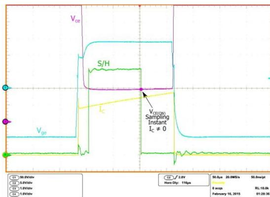
Figure 5. Double pulse test shows waveforms of current  $I_c$  gate-emitter voltage  $V_{ge}$ , collector-emitter voltage  $V_{CE}$  and sampling signal S/H
