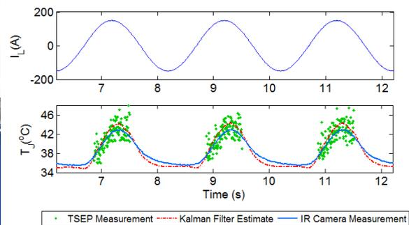
Figure 12. Experimental real-time measurements of loading current  $I_L$  and the corresponding  $T_J$  measurement from TSEP and IR Camera compared to the  $T_J$  estimate given by Kalman Filter.
