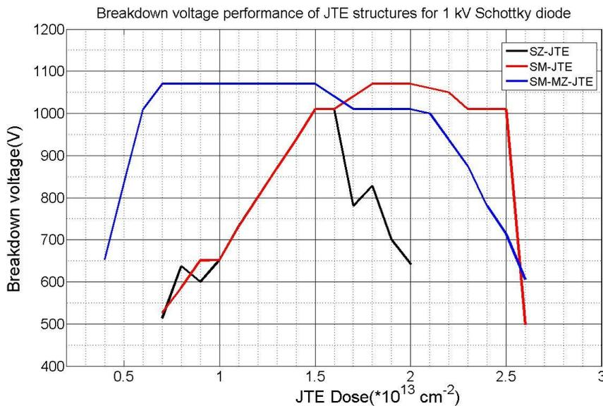
Fig.6. Simulated JTE dose dependence of breakdown voltage for 1kV Schottky diode with different JTE structures.
