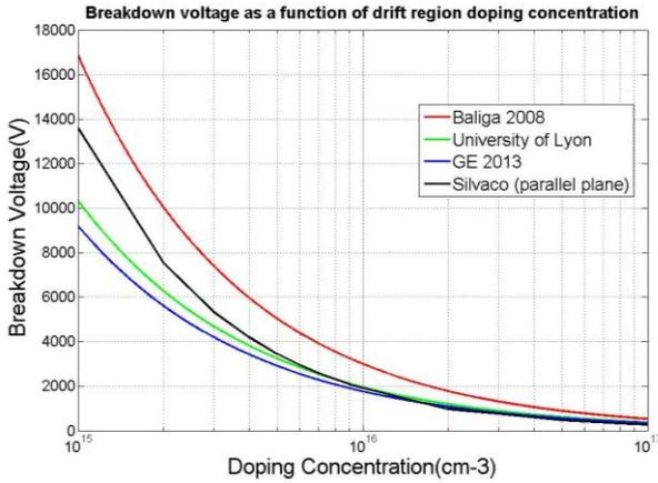
Fig.2. Breakdown voltage versus doping concentration of 4H-SiC for different
