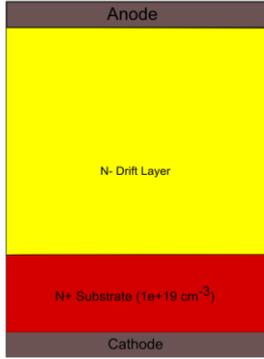
Fig.1. Schematic of parallel plane Schottky
