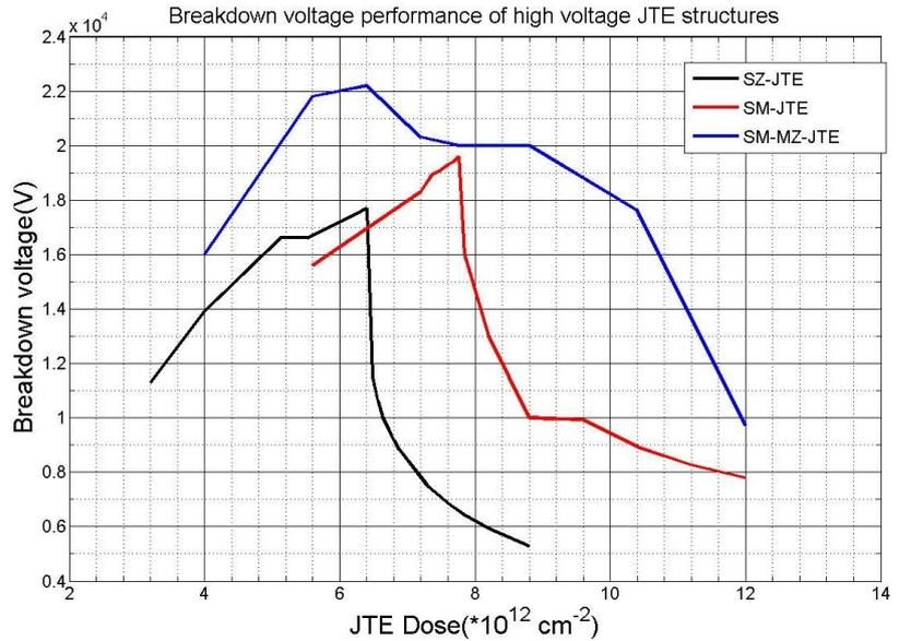
Fig.5. Simulated JTE dose dependence of breakdown voltage for 22.5 kV PiN diodes with different JTE structures.
