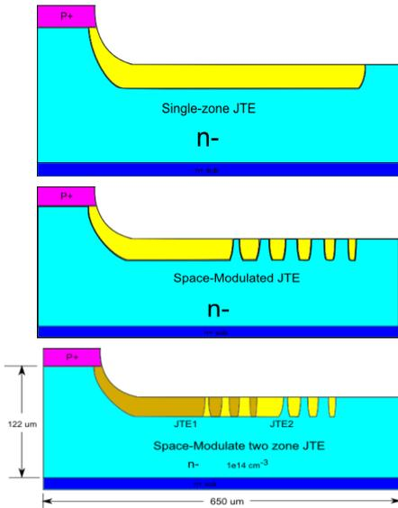
Fig.4. Schematics of the three different JTE structures of PiN
