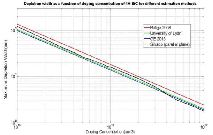
Fig.3. Depletion width versus doping concentration (both in log scale) of 4H-SiC for different estimation methods.
