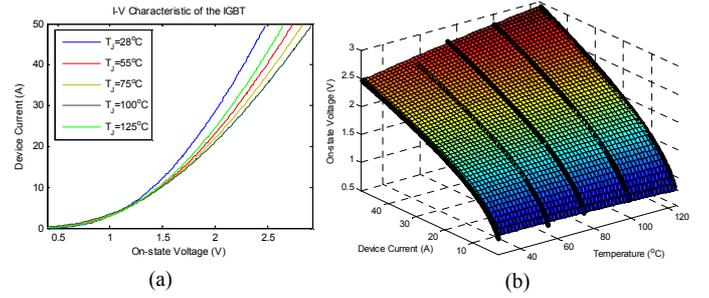
**Figure 4** (a) the I-V characteristic of an IGBT device (b) the electrical model of an IGBT device
