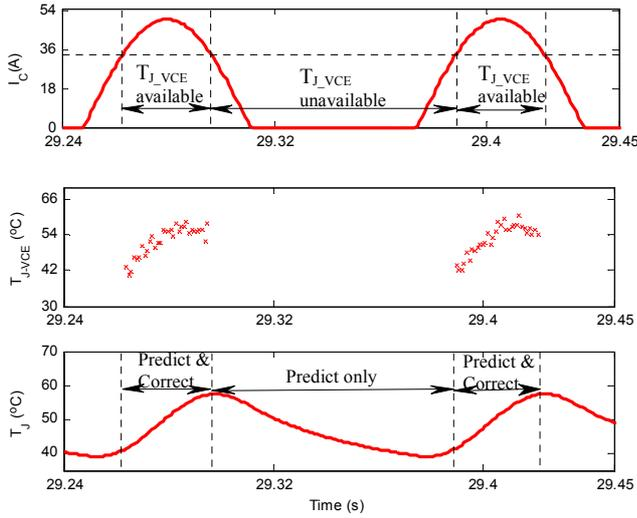
**Figure 6** availability of the estimate  $T_{J\_VCE}$  and the corresponding steps of Kalman filter
