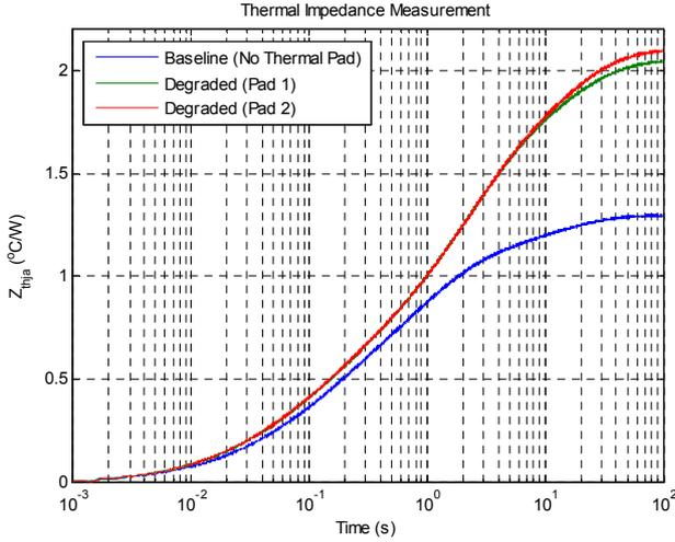
**Figure 3** Experimental thermal impedance measurements of Baseline and Degraded IGBT module
