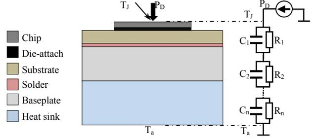
**Figure 1** the multilayer structure of a power module and its equivalent foster network
