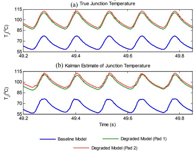
**Figure 8 (a)** True junction temperature **(b)** Kalman Estimate of junction temperature
