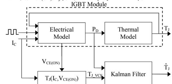
**Figure 5** The Electro-Thermal Simulink model
