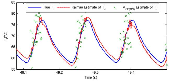
**Figure 7** Kalman Estimate of  $T_j$  compared to True  $T_j$  and  $V_{CE(ON)}$  estimate  $T_{J\_VCE}$
