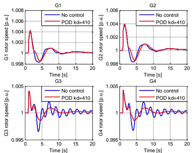
Fig. 12. Generator rotor speed responses to a three-phase fault with and without supplementary VSC-HVDC POD controller
