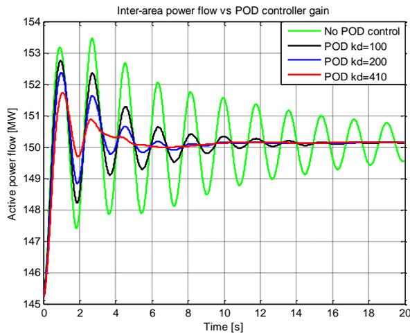
Fig. 11. Inter-area active power flow (line 3) responses to the small signal disturbance for a range of POD controller gains
