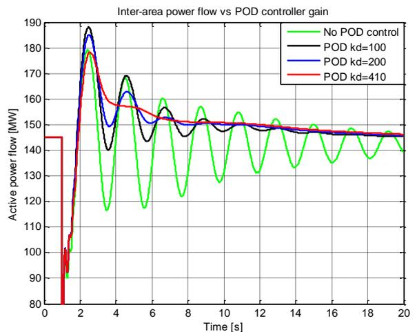
Fig. 13. Inter-area active power flow (line 3) responses to a three-phase fault for a range of POD controller gains
