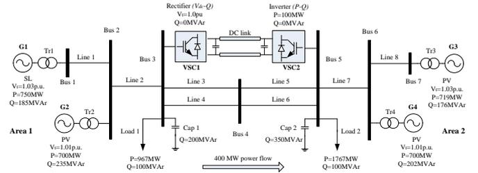
Fig. 5. Four-machine two-area test system incorporating VSC-HVDC transmission
