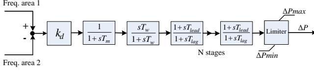
Fig. 7. Block diagram of a feedback power oscillation damping controller
