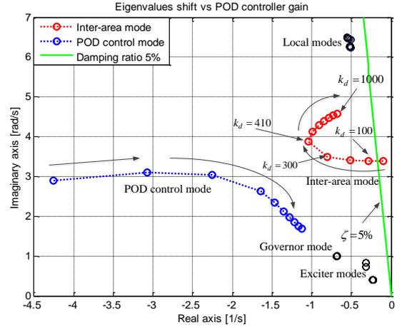
Fig. 9. Oscillatory modes versus the gain of the VSC-HVDC POD controller
