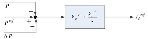
Fig. 3. Active power control loop
