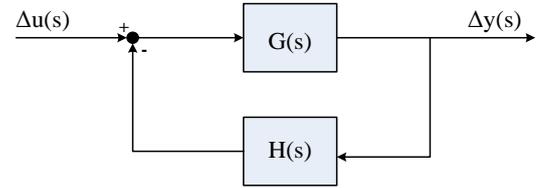
Fig. 6. Closed-loop system with POD feedback control
