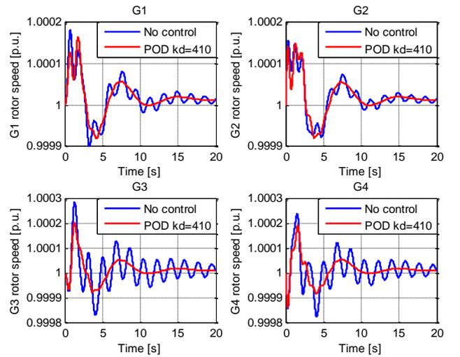
Fig. 10. Generator rotor speed responses to the small signal disturbance with and without supplementary VSC-HVDC POD controller
