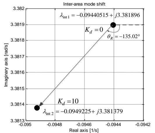
Fig. 8. Residue's phase angle estimation for POD controller design
