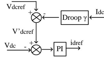
Fig.4: Modifications of Vdcref in Vdc-Q control of a slack converter.
