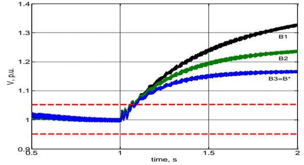
Fig. 6a: Vdc in the DC grid for different values of  $\beta$ . Voltage limits (+1.05, -0.95) shown in red.
