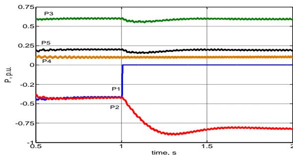
Fig. 7b: Converter power flows for  $\beta=\beta^*$  and  $\gamma=\gamma^*$  (+ means injected power, - exported power).
