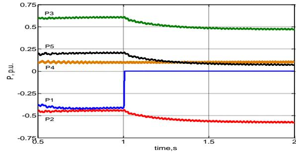
Fig. 6b: Converter power flows for  $\beta=B^*$  (+ means injected power, - exported power).
