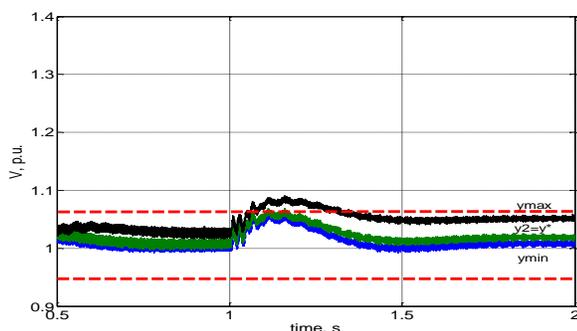
Fig. 7a: Vdc in the DC grid for different values of  $\beta$ . Voltage limits (+1.05, -0.95) shown in red.
