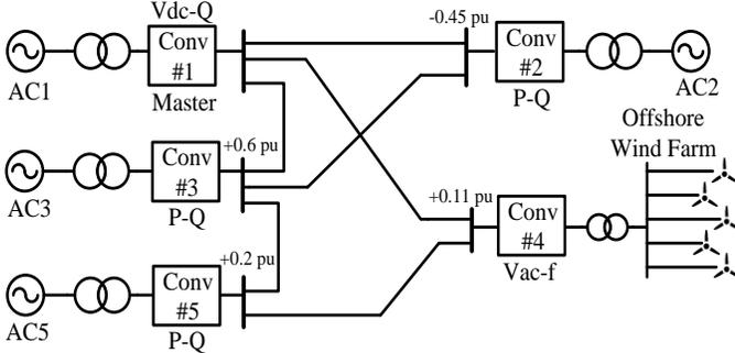
Fig. 5: 5-terminal DC grid model developed in RT-Lab Simulator.
