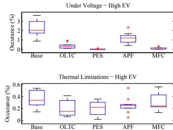
Fig. 13. Network with 71% proliferation of Electric Vehicles
