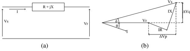
Fig. 2. Network power flow (a) and associated phasor diagram (b)
