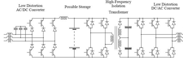
Fig. 3. Possible Configuration of a PES
