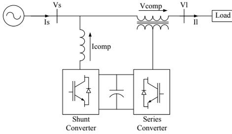
Fig. 6. Configuration of a UPQC
