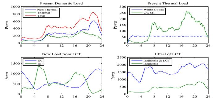
Fig. 8. Top Left: Average Domestic 24 hour demand profiles. Top Right: Thermally Controlled Loads (White Goods & Restive Based). Bottom Left: EV and HP loads. Bottom Right: Present Load Profile and with 100 % LCT use
