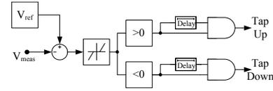
Fig. 4. AVC Type Control Logic of an OLTC
