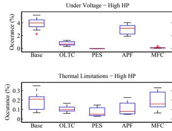
Fig. 11. Network with 80% proliferation of Heat Pumps
