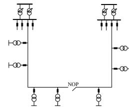
Fig. 1. Typical Arrangement of HV radial network with interconnected normally open point (NOP) for security of supply
