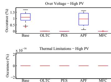
Fig. 15. Network with 60% proliferation of PV Installations
