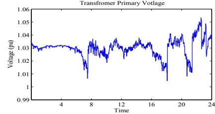
Fig. 7. Voltage Profile at Primary Side of the LV Substation
