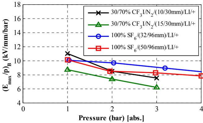
Fig. 9: Pressure-reduced maximum breakdown field strength,  $(E_{\max}/p)_B$ , as a function of pressure for SF<sub>6</sub> and 30/70% CF<sub>3</sub>I/N<sub>2</sub> for coaxial test systems with geometric ratios of 1/2 and 1/3 and for positive lightning impulse.
