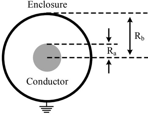
Fig. 2: Cross-section view of a coaxial geometry.
