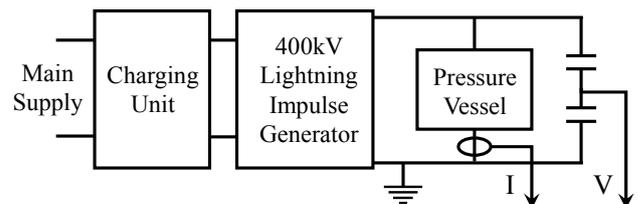
Fig. 1: Test circuit for standard 1.2/50 lightning impulse breakdown tests.
