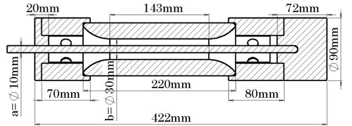
Fig. 4: Design of reduced-scale coaxial GIL test system. The values of "a" and "b" indicate the diameters corresponding to  $R_a$  and  $R_b$ .
