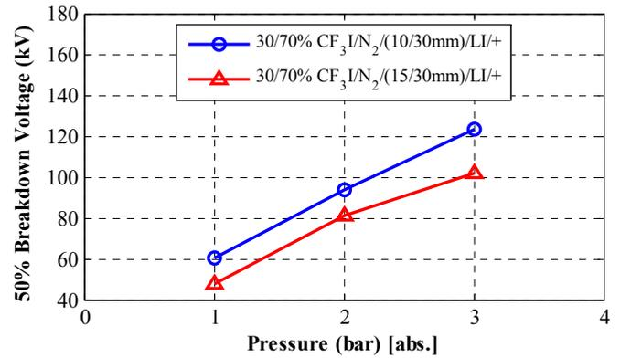
Fig. 8: Breakdown voltage,  $U_{50}$ , for 30/70% CF<sub>3</sub>I/N<sub>2</sub> gas mixture at pressure range of 1 to 3 bar (abs.) for different diameters of the inner conductor in the coaxial test configuration for positive lightning impulse.
