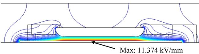
Fig. 6: Plot of electric field distribution showing the maximum electric field at the center of the conductor.
