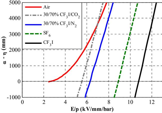
Fig. 5: Effective ionisation coefficients in pure gases (Air, SF<sub>6</sub> and CF<sub>3</sub>I), and gas mixtures (30/70% CF<sub>3</sub>I/N<sub>2</sub> and 30/70% CF<sub>3</sub>I/CO<sub>2</sub>).
