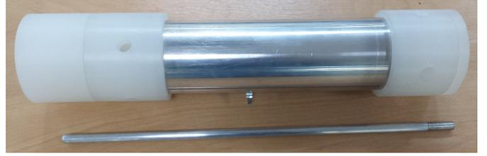
Fig. 7: Photograph of the reduced-scale coaxial test system.
