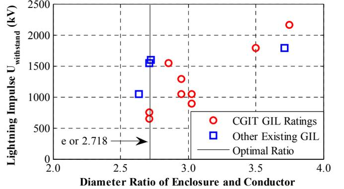
Fig. 3: Relationship between lightning impulse withstand voltage and dimensions in existing GIL systems.
