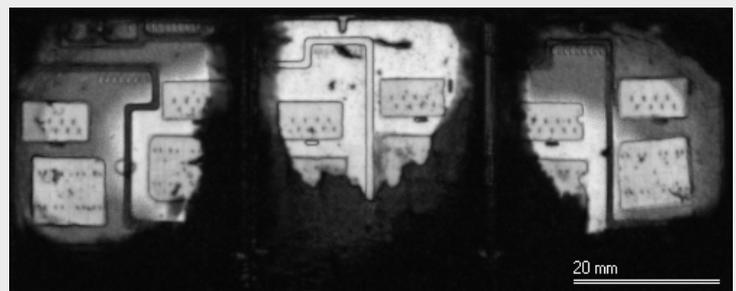
Scanning Acoustic Microscopy (SAM) of an IGBT power module. Top image shows the module in as received pristine conditions where the substrate copper and semiconductor devices can be seen. Bottom image shows the same module after 17500 cycles of power cycling test. The black shadow indicates a delamination in the substrate solder layer due to solder fatigue mechanism.
